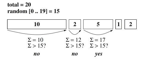
Each process is assigned a number of tickets (single integer in PCB). When the scheduler is triggered, a random ticket number in the range between 0 and the total number of tickets is generated. The scheduler than iterates over the list of ready processes and adds up each process's ticket amount. If the sum becomes greater than the chosen random ticket, the current process must own the ticket and the lottery scheduler consequently selects it for dispatching.
